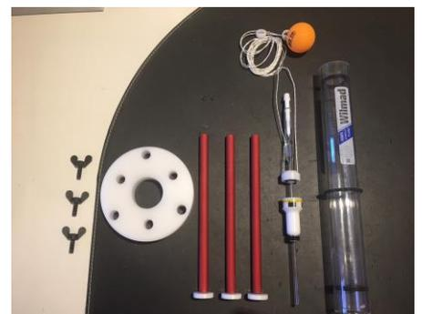
Fig. 3, Parts from left to right: Screws, white support ring, rods, pressure tube inserted in tube holder and spinner turbine, tube assembly.
